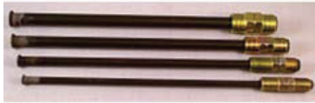
Figure 4. Steel gas lines in various diameter used for burning the craters.
