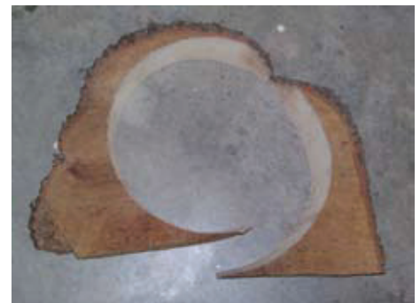
This photo shows the amount of shrinkage from when the blank was cut from the block of wood.
