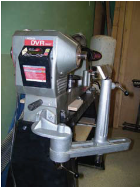
This photo shows the Nova Outrigger mounted to the lathe bed and in position for turning.
