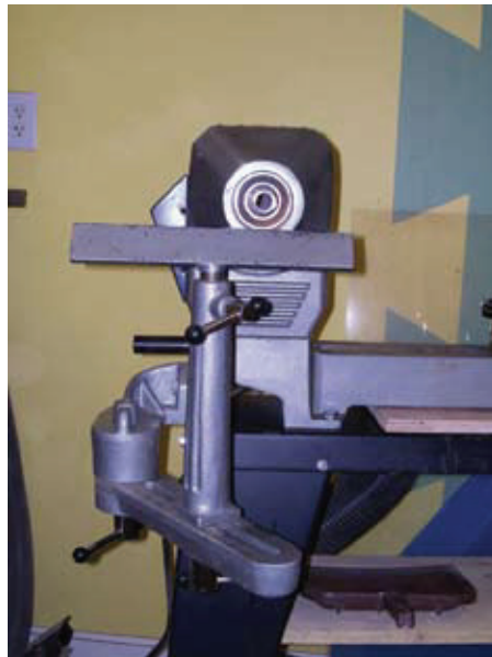
Front view of the lathe with outrigger in position to turn wood.
