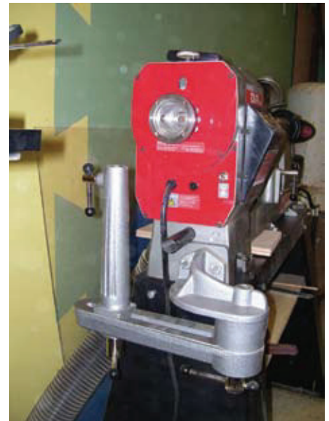
This view shows the outrigger stored in position at the end of the lathe bed. It is out of the way for normal turning.
