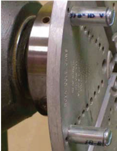
Figure 4. Shows the upgrade installed and seems to hold the piece a little more securely than the rubber buns provided with the Cole Jaws.
