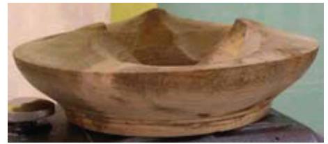
Figure 2. This photo shows a triple off-center turned bowl and its edge does not sit on the Cole plates resulting in no edge to grip with the buns.
