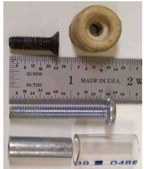
Figure 3. This photo shows the components needed to upgrade the Cole Jaws capacity.
