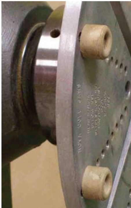
Figure 1. This photo shows the rubber buns have a height of 1/2" and work well with conventional edge bowls.
