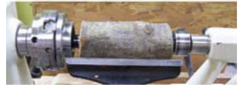
Figure 3. Wood for the handle mounted between centers to turn a tenon to fit into the chuck.
