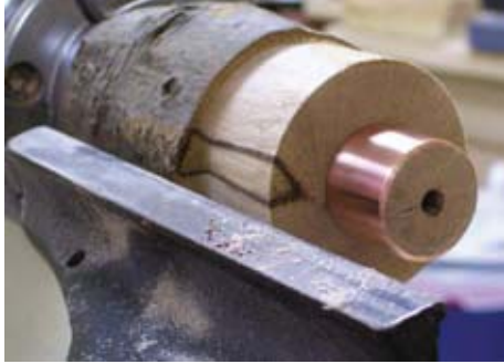
Figure 4. Here the collar has been fitted to the wood.
