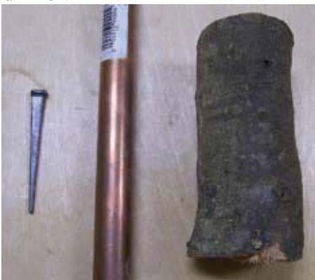
Figure 1. Materials consist of a Masonry Nail, a piece of copper tubing, and wood for the handle.
